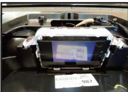
1. Remove 2 screws holding OEM screen in place
