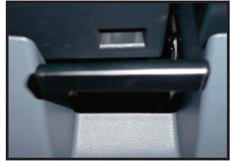
3. Use lever to drop steering wheel column down
