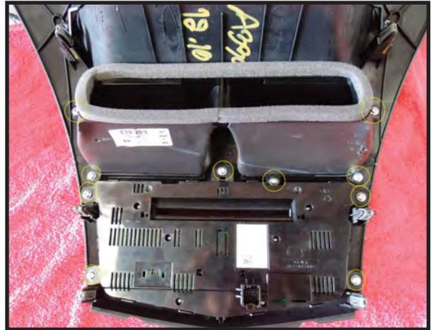
2. Remove the 10 screws holding the button panel and air conditioning vents in place - set aside.
