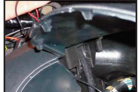
8. You can now remove the tape and feed the Bluetooth mic cable into the TOP SECTION
