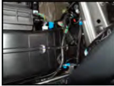
2. Unclip OEM USB and AUX cable for now, so that you can remove the glove box completely.
