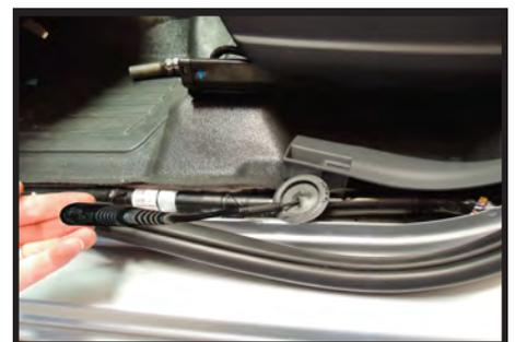
10. Use cutters to make an incision in grommet so that you feed cable through it. Once you have fed the cable through the grommet restore grommet back into its original position.
