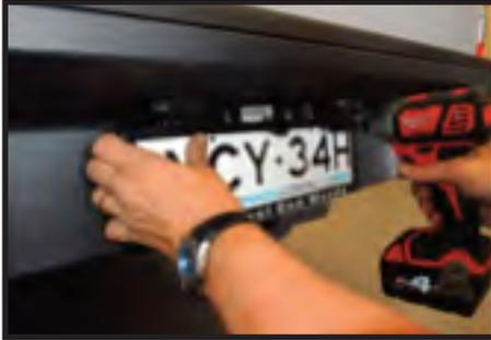
5. Mount number plate back onto the vehicle.
