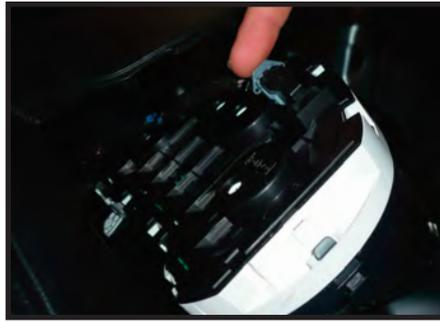
13. Plug harness back into instrument cluster panel and remount.
