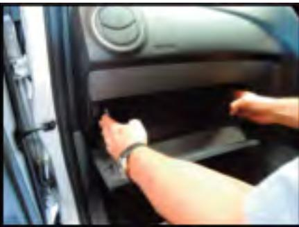
1. Remove glove box - gently push in sides to release.
