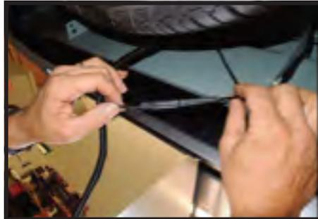
6. Connect camera plug to the extension cable. Apply heat shrink over connection to avoid the plug coming loose.
