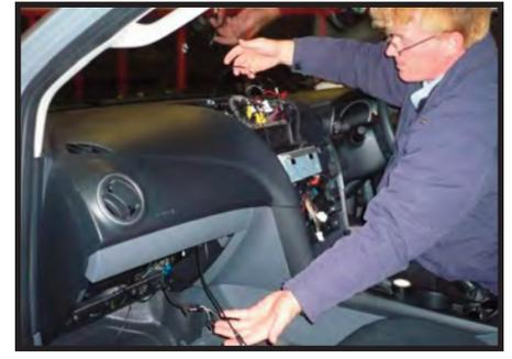
3. Feed RW50/15 USB cable from top section down into the glove box area
