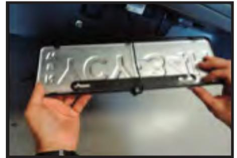
4. Attach the number plate camera onto number plate (as shown above)
