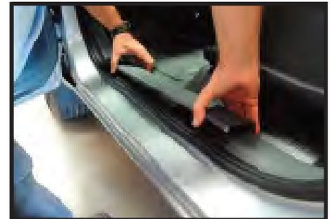
7. Remove kick panel and scuff plate on passenger front side of vehicle
