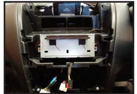
3. Remove 2 screws holding the CD housing in place.
