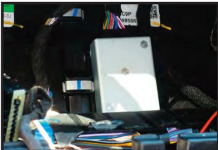
1. Before re-mounting the OEM CD Housing we suggest positioning the power amplifier box just behind it.
