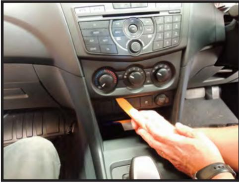
1. Starting from the bottom, use trim tools to remove air conditioning controls
