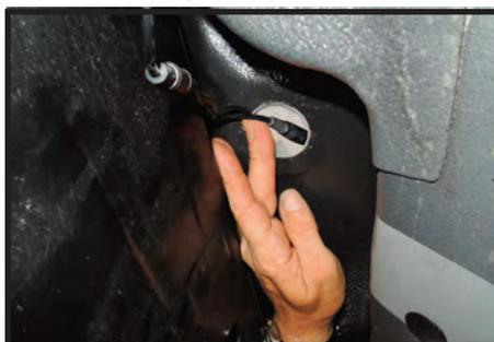
9. Remove grommet and feed cable through
