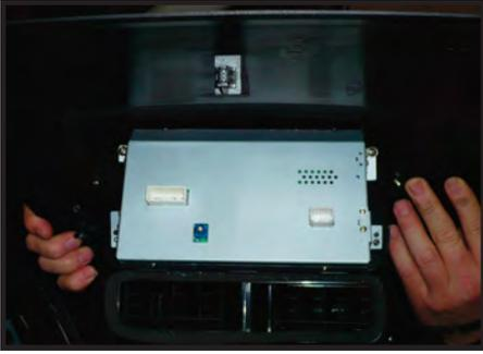
1. Connect PLUG B & E into the back of the RW50/15 interface screen
