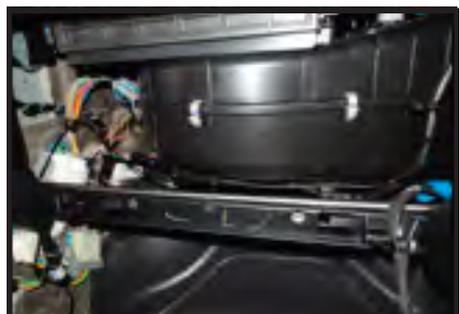
12. Run reverse camera cable up into glove box area.
