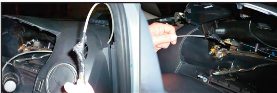
7. Tape Bluetooth mic cable onto strike and pull through to the instrument cluster panel area
