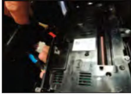
2. Plug the OEM button panel harness into the back of the OEM button panel
