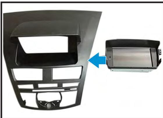
5. Use the 2 screws to attach the RW50/15 screen to the fascia.
