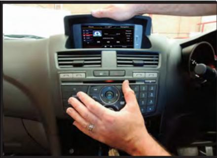
4. Rest the unit in place, test all features first and then gently push fascia panel back into position
